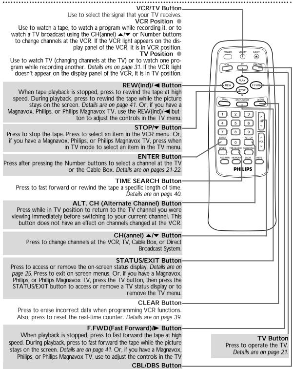
Press to operate the Cable Box or Direct Broadcast System. Details are on page 22.
